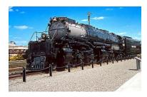
Meet the Big Boy, the largest successful locomotive engine ever created. They were built for one purpose and one purpose alone: to pull large tonnage over the 1.55% continuous grade up Sherman Hill in the Wasatch mountain region just east of Ogden Utah. Each Big Boy with its tender weighed 1,208,750 lb.
