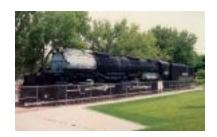
Meet the Big Boy, the largest successful locomotive engine ever created. They were built for one purpose and one purpose alone: to pull large tonnage over the 1.55% continuous grade up Sherman Hill in the Wasatch mountain region just east of Ogden Utah. Each Big Boy with its tender weighed 1,208,750 lb.
