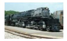
Meet the Big Boy, the largest successful locomotive engine ever created. They were built for one purpose and one purpose alone: to pull large tonnage over the 1.55% continuous grade up Sherman Hill in the Wasatch mountain region just east of Ogden Utah. Each Big Boy with its tender weighed 1,208,750 lb.
