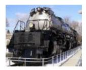
Meet the Big Boy, the largest successful locomotive engine ever created. They were built for one purpose and one purpose alone: to pull large tonnage over the 1.55% continuous grade up Sherman Hill in the Wasatch mountain region just east of Ogden Utah. Each Big Boy with its tender weighed 1,208,750 lb.
