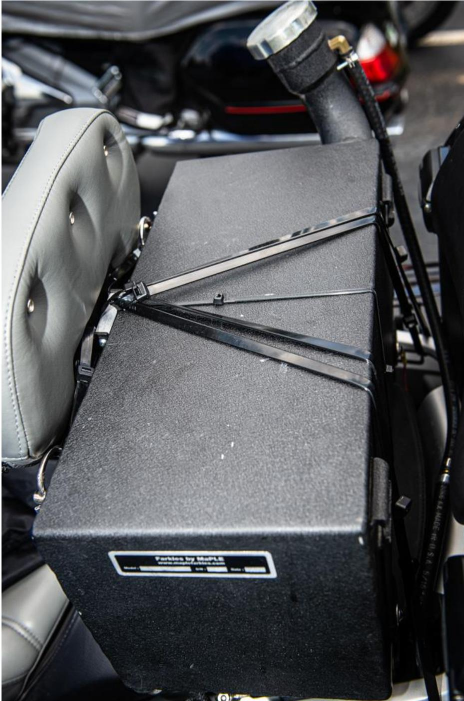
Fortunately, the world has not spun off its axis. Jim's cell was properly bolted and secured to the subframe. The zip ties have nothing to do with tank mounting and are used to stabilize his back rest in the proper position. As one would expect, Jim's bike passed tech just fine, but we are not done mentioning Jim in this daily report.
